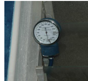
Sphygmo as a tank level gauge
