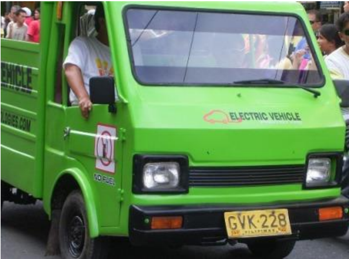
This is one of the most popular small vehicles in the province, called the “EZ Ride”. Obviously, in this case, the engine was replaced by an electric motor with huge battery pack making the bigger payload.
