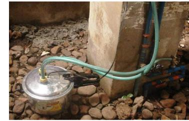
Pressure cooker as enclosure for solar fish-tank pump, 15 watt
