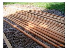
What gu-od looks like, short and thick, versus regular bamboo above, and finally coco (coconut) lumber.
